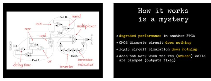
Here are some strange things about the circuit. Recall that the training / evolution process used an actual FPGA; when a different physical part is substituted for the one trained on, the circuit doesn't work as well—the evolution was particular to the physical part that was used. If you make the circuit in the diagram with CMOS, it doesn't work. If you simulate the circuit with one of the commercial simulators, it does nothing.
